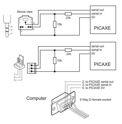
Note that the two resistors are not a potential divider. The 22k resistor works with the internal microcontroller diodes to clamp the serial voltage to the PICAXE supply voltage and to limit the download current to an acceptable limit. The 10k resistor stops the serial input 'floating' whilst the download cable is not connected. This is essential for reliable operation.
