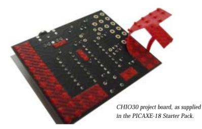
This peelable layer protects the user solderable pads during manufacture and storage, to keep the pads clean and grease free.
