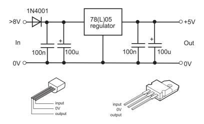
**IMPORTANT NOTE** - this manual describes use of the standard range (3-5V) parts. The X2 parts are also optionally available in special low power (1.8V to 3.3V) variants. Use of a 5V supply on a 3.3V part will permanently damage it!
