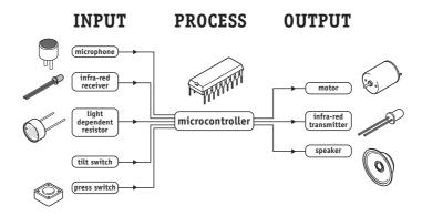
The microcontroller uses information from the input transducers to make decisions about how to control the output devices. These decisions are made by the control program, which is downloaded into the microcontroller. To change the 'behaviour' of the toy it is simply a process of changing and downloading a new program into the microcontroller
