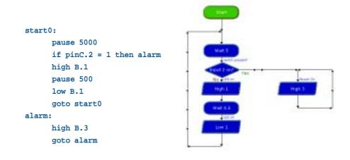
The student's first attempt at programming is shown in flowchart 1 above. This is the obvious solution, but does not work as expected. This is because the alarm does not sound immediately when the wire is cut - as the input is only checked once every 5 second there can be up to 5 seconds 'lag' before the alarm sounds.
