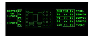
Pins 3 and 4 include on-board 10k pull down resistors so that these pins may be used directly as inputs without any other modification.
