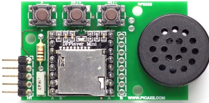
The SPE035 Serial MP3 player consists of a small MP3 player module mounted on a PCB with serial connector, test switches and 8 ohm speaker. It provides a simple and low cost way to add MP3 tune playback to any PICAXE project.
