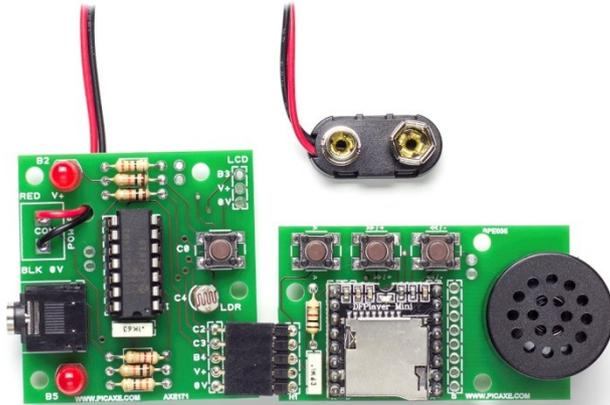
The following examples assume use of the AXE171 PICAXE 14 Audio Kit, so if using a different board you may need to alter the input / output pins in these examples (which are 'serial transmit' on output B.4 and 'busy signal' receive on input pinC.2).
