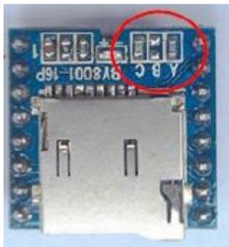
The PCB is also compatible with the 'BY8001-16P' module. This is used in position 'B' as it has a different size/pinout. Note that for serial control of the BY8001 it **must** be put into 'serial mode 111' by **removing all 3** resistors shown in the red circle (the default is normally a resistor in positions 'A' and 'C' with 'B' already removed).
