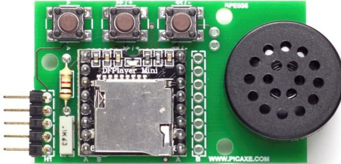
Note that there are two positions (A or B) on the PCB for the MP3 player module. This is because MP3 playback modules using the YX5300 MP3 chip are available in various different types and sizes. Carefully check the position of your module before soldering on to the board.
