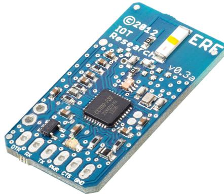
The ERF is the easiest and most convenient way to wirelessly communicate between a PICAXE chip and a computer, or between 2 (or more) PICAXE chips.
