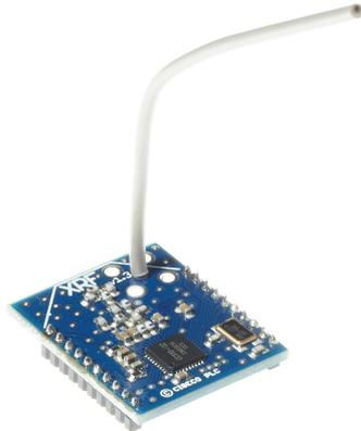
The XRF is an XBee footprint compatible module to allow wirelessly communication between a PICAXE chip and a computer, or between 2 (or more) PICAXE chips. The XRF transparently passes serial characters to and from individual or multiple radio devices. You don't need to use complex encoding or error checking as it is all done for you - simply send raw text/data via 'serout', and receive text/data via 'serin'.
