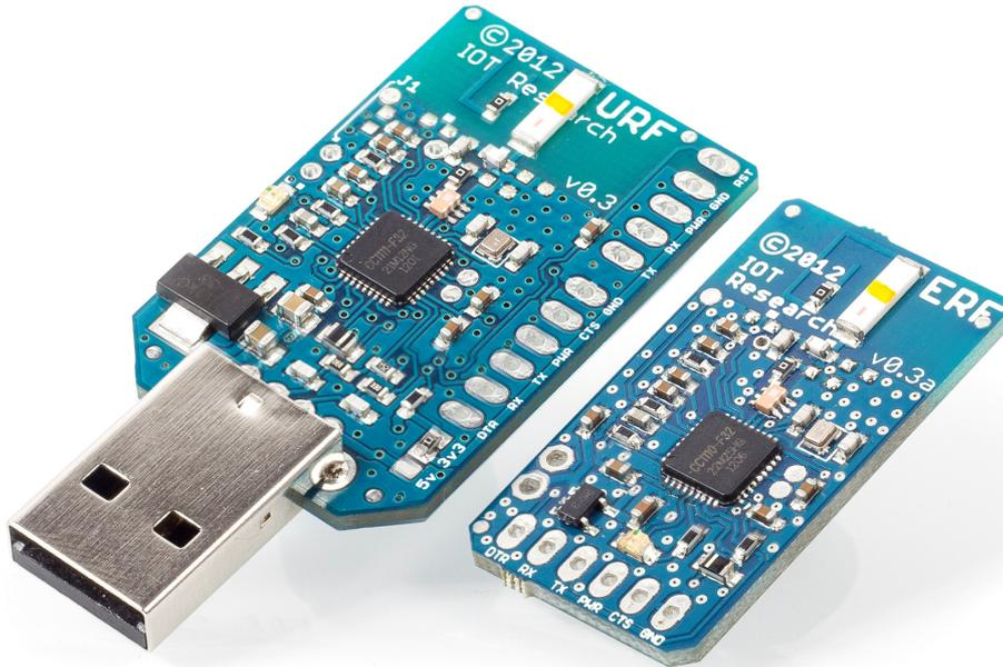
The ERF, URF and XRF modules are designed to provide ‘out-of-the-box’ instant wireless bi-directional serial communication between a computer and/or multiple PICAXE project boards. All 3 modules are designed around the Texas Instruments CC111x combined micro & RF transceiver integrated circuit.
